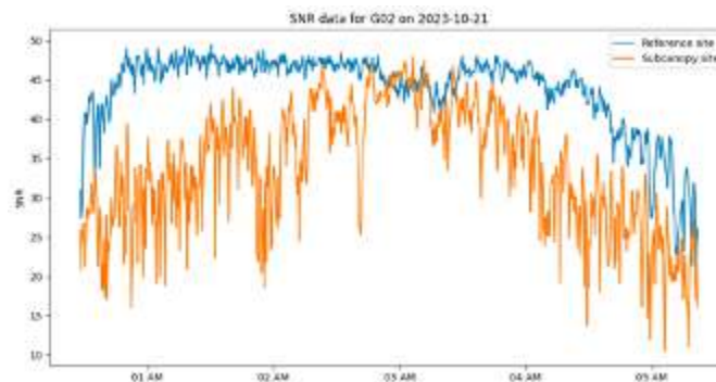
Figure 1. Graph depicting the fluctuation in signal-to-noise ratio of satellite G02 between a reference and subcanopy site on a sub-daily scale during October 21st, 2023.
